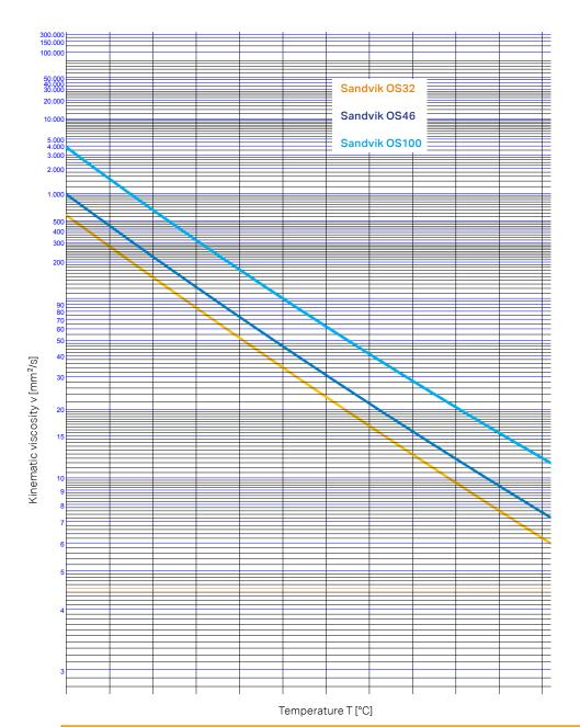
The diagram makes it easy for the user to find the correct viscosity grade for your working temperature.
