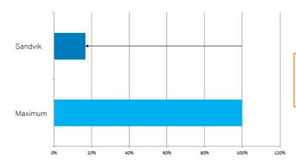
Sandvik OT220 shows excellent results in FE8 roller wear tests and reduces wear in your bearings up to 80 %.
