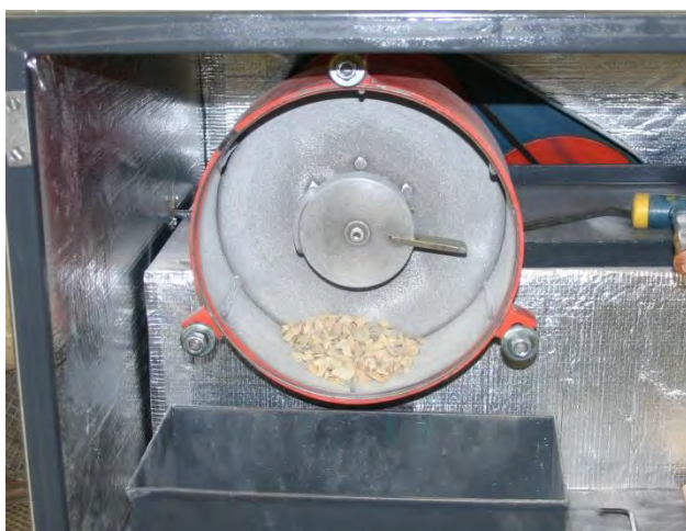
Test apparatus for determination of Abrasion Index (AI) along with test paddle before and after test.
