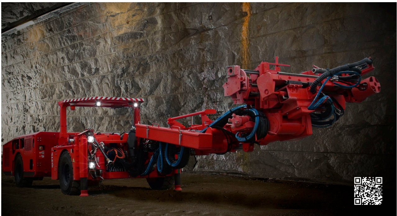
1. SANDVIK DS211L-M - LOW PROFILE BOLTER
