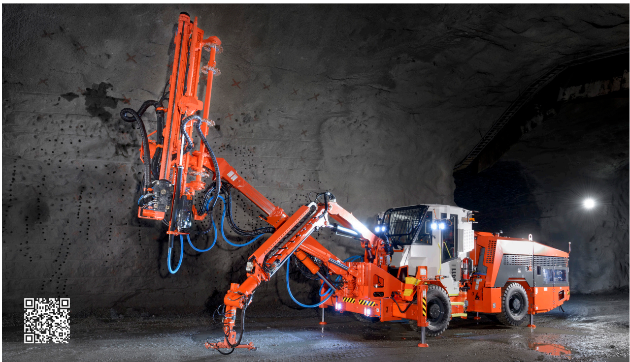
1. SANDVIK DS411 - ROCK SUPPORT BOLTER
