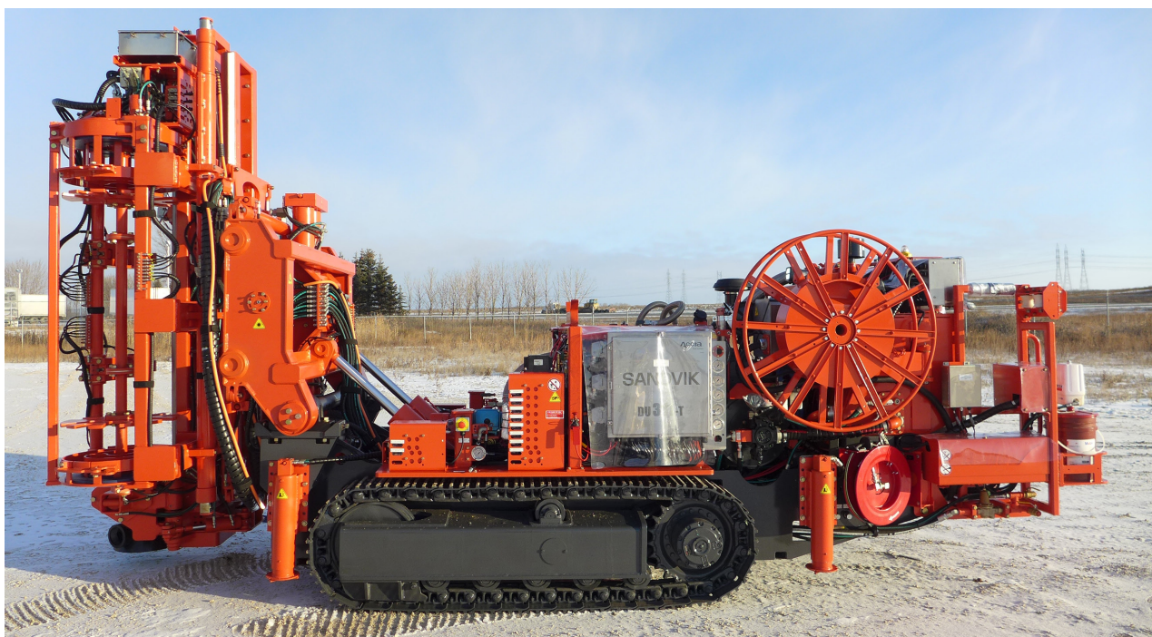
1. SANDVIK DU311-TK - ITH LONGHOLE DRILL
