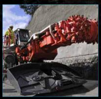
ROADHEADERS AND CUTTING UNITS Sandvik roadheaders are extremely powerful rock-cutting machines designed to excavate roadways, tunnels and chambers continuously without using explosives. Their ability to excavate the desired profile without causing harmful vibrations is highly valued for both environmental and safety reasons. The roadheader family also includes multi-purpose hydraulic-driven cutting heads for mounting on excavators.
