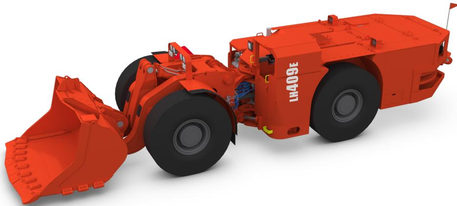
The LH409E is an electrically-driven loader for underground hard rock loading and hauling applications, with a tramming capacity of 9.6 metric tonnes. Reliability, fast bucket filling and rapid cycle times provide high capacity at low cost per tonne. The LH409E fits in an envelope of 3.5 m x 3.5 m.
