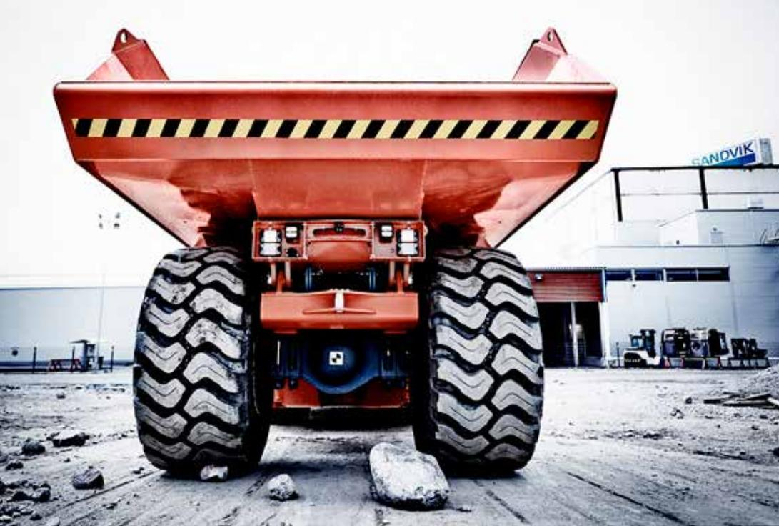
The envelope sizes are made for 5x5- and 6x6-metre haulage ways.
