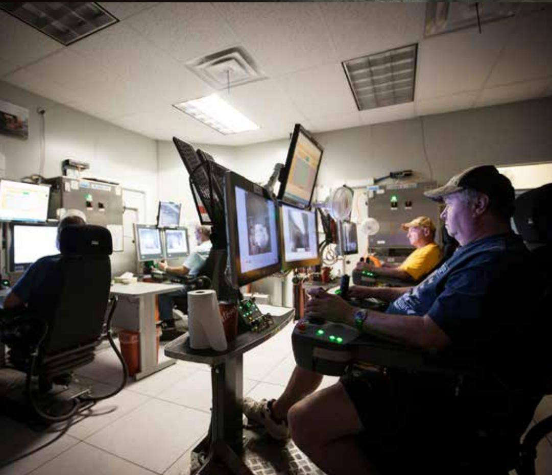
**USING AUTOMATED LOADERS** adds complexity to the operation. Areas where automated loaders are tramping need to be closed off to personnel – in some existing mines, such as Kidd Operations, this can mean securing an entire level – and mechanics need to be trained in automated components. Despite these complexities there are clear benefits, Roberts says.
