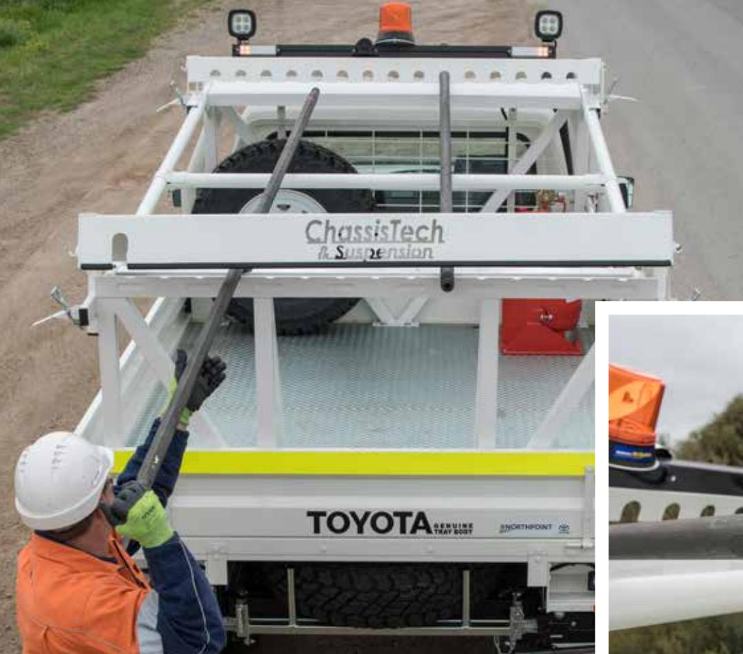
The rods are double-clamped and strapped down to ensure secure transport.
