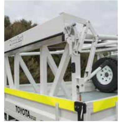
The new design enables personnel to safely transport drill rods without their sliding around or falling off the vehicle.
