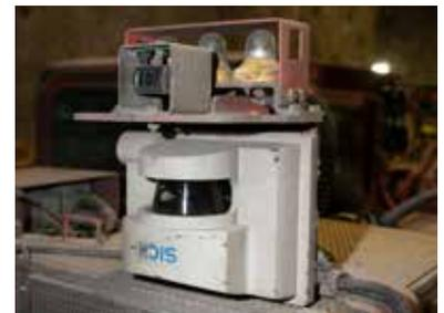
**Seven onboard cameras and two scanners show the operators above ground what is going on all around the loader and enable them to intervene, if necessary.**
