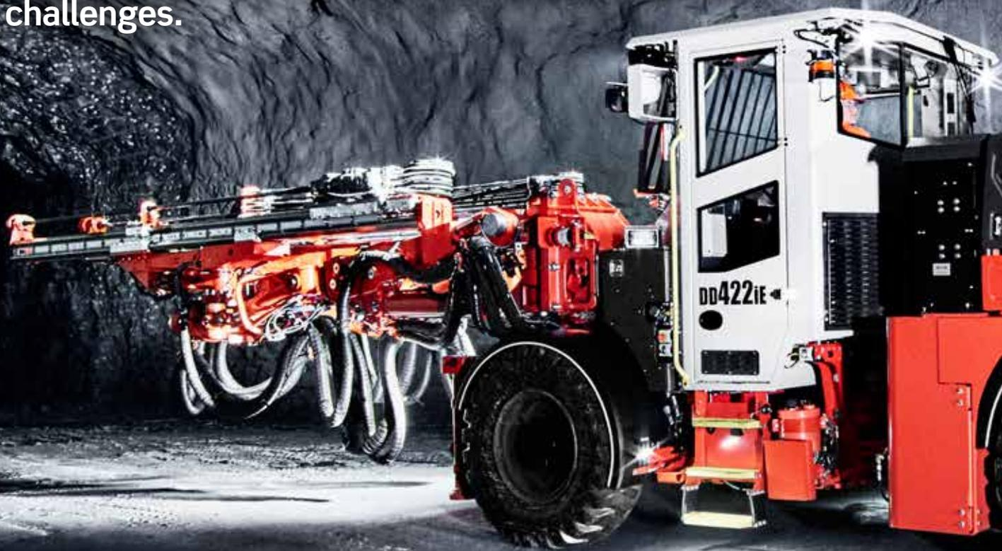
▶ **AS REGULATIONS BECOME** stricter, mines need cleaner-energy solutions that help reduce DPM emissions in their underground operations. Replacing diesel equipment with battery-driven versions helps eliminate such contaminants and associated respiratory risks while reducing operating costs.
