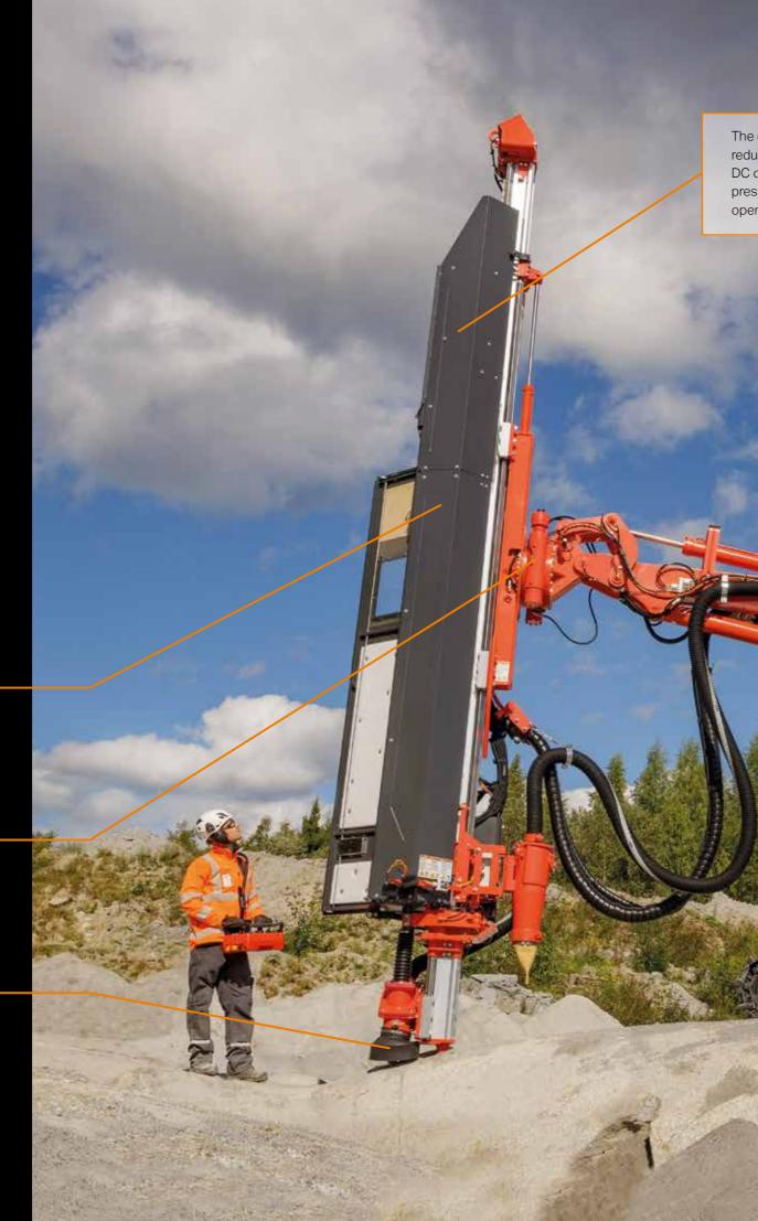
The optional NoiseShield-DC is a simple and compact noise reduction solution for the Dino<sup>™</sup> DC410Ri. The NoiseShield-DC offers up to a -7.5 dB reduction in A-weighted sound pressure by directing the drilling noise upwards through an open top, away from the operator and surrounding areas.
