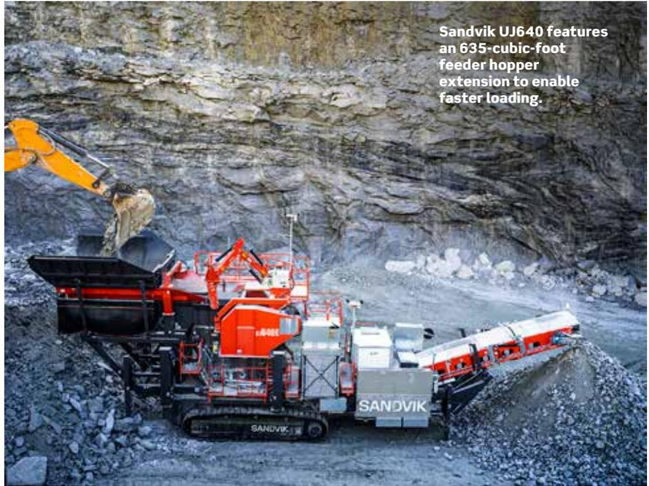
Sandvik UJ640 features an 635-cubic-foot feeder hopper extension to enable faster loading.
