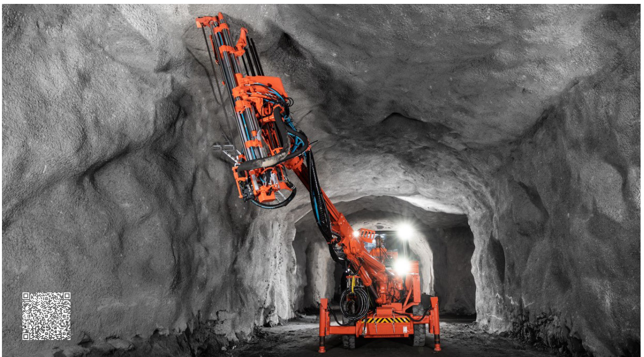
1. SANDVIK DS311D - ROCK SUPPORT BOLTER
