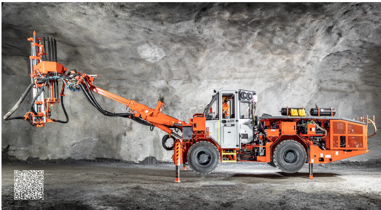
1. SANDVIK DS311DE - ROCK SUPPORT BOLTER
