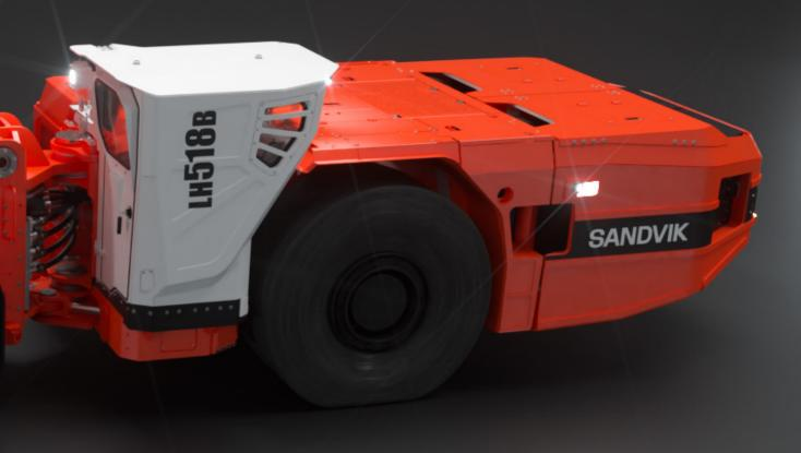
s equipped with a unique patented self-swapping system a Battery swapping with the ast and easy and with minimum nual handling. The AutoSwapire any mine infrastructure swaps, and it is faster than traditional diesel loader.
