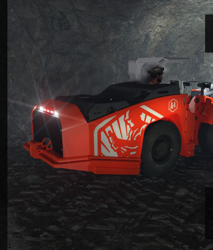
The A4 produces zero diesel emissions thereby reducing demand on your mine's ventilation and cooling systems making deep mining possible. It improves working conditions and enables the incalculable benefits of a healthier underground environment.
