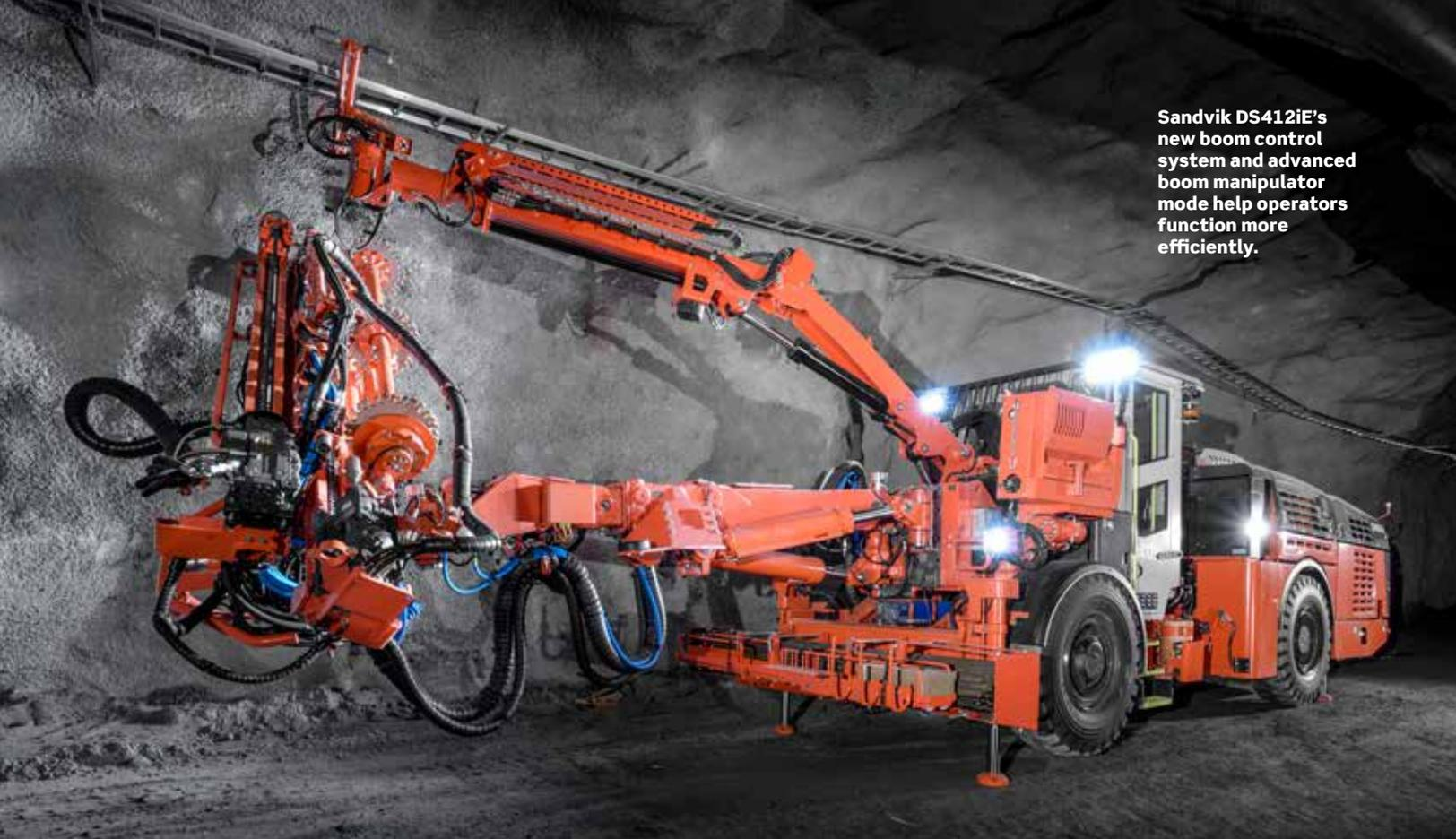
Sandvik DS412iE's new boom control system and advanced boom manipulator mode help operators function more efficiently.
