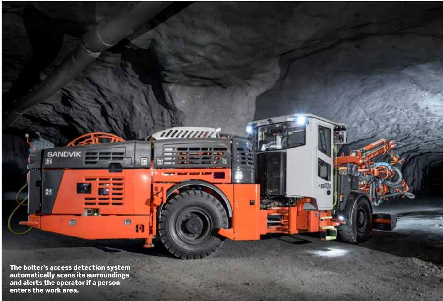
The bolter's access detection system automatically scans its surroundings and alerts the operator if a person enters the work area.
