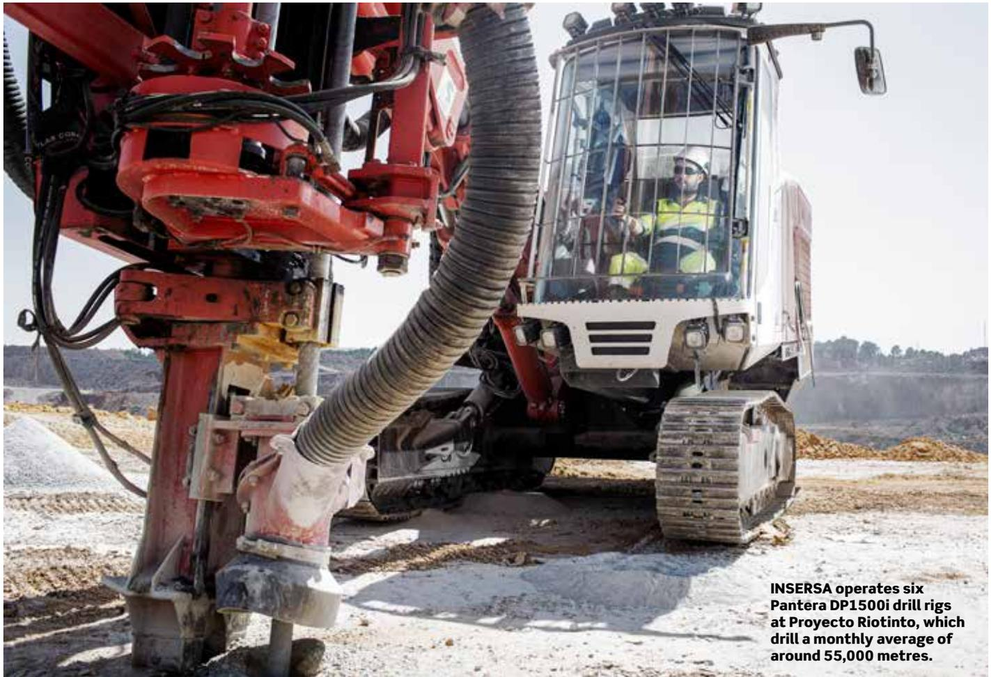
**INSERSA operates six Pantera DP1500i drill rigs at Proyecto Riotinto, which drill a monthly average of around 55,000 metres.**
