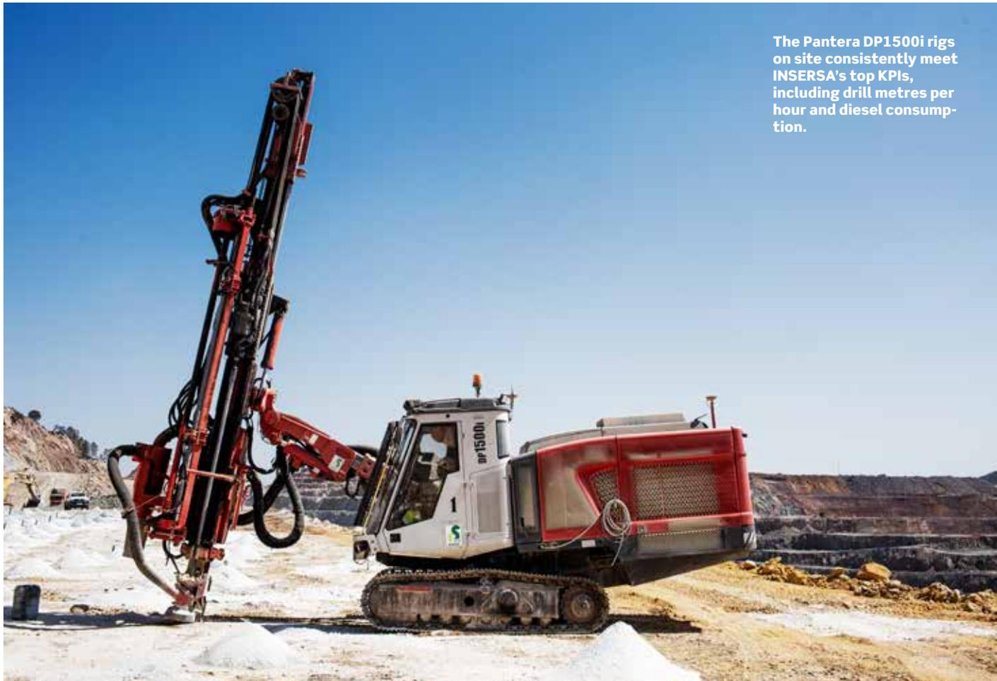
The Pantera DP1500i rigs on site consistently meet INSERSA's top KPIs, including drill metres per hour and diesel consumption.
