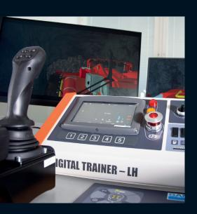
The Portable version of the Digital Trainer – LH, training simulator for the  $\mathsf{Toro}^\mathsf{TM}$  LH517i and  $\mathsf{Toro}^\mathsf{TM}$  LH621i loaders, offers an efficient and flexible tool for operator training. The Portable Digital Trainer allows to start practicing loader operation well before the actual loader arrives to the site, leaving the on-site equipment available for productive work. The Portable Digital Trainer significantly improves the overall training efficiency.
