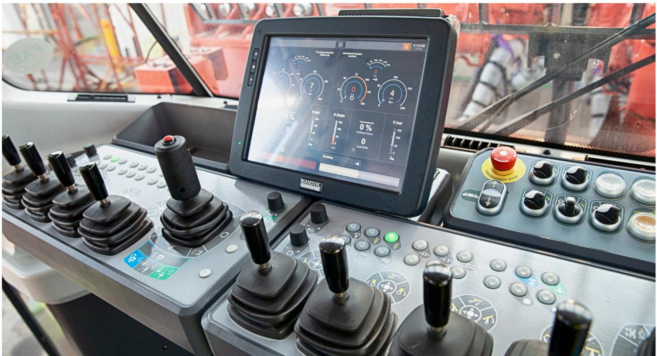
1. SANDVIK DUAL DRILLING CONTROLS - DEVELOPMENT DRILLS
