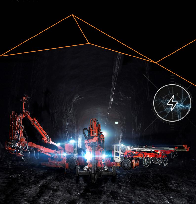
Sandvik comprehensive battery-powered range for drift sizes 4 by 4 meters and up, is available for all underground drilling applications and most mining methods.
