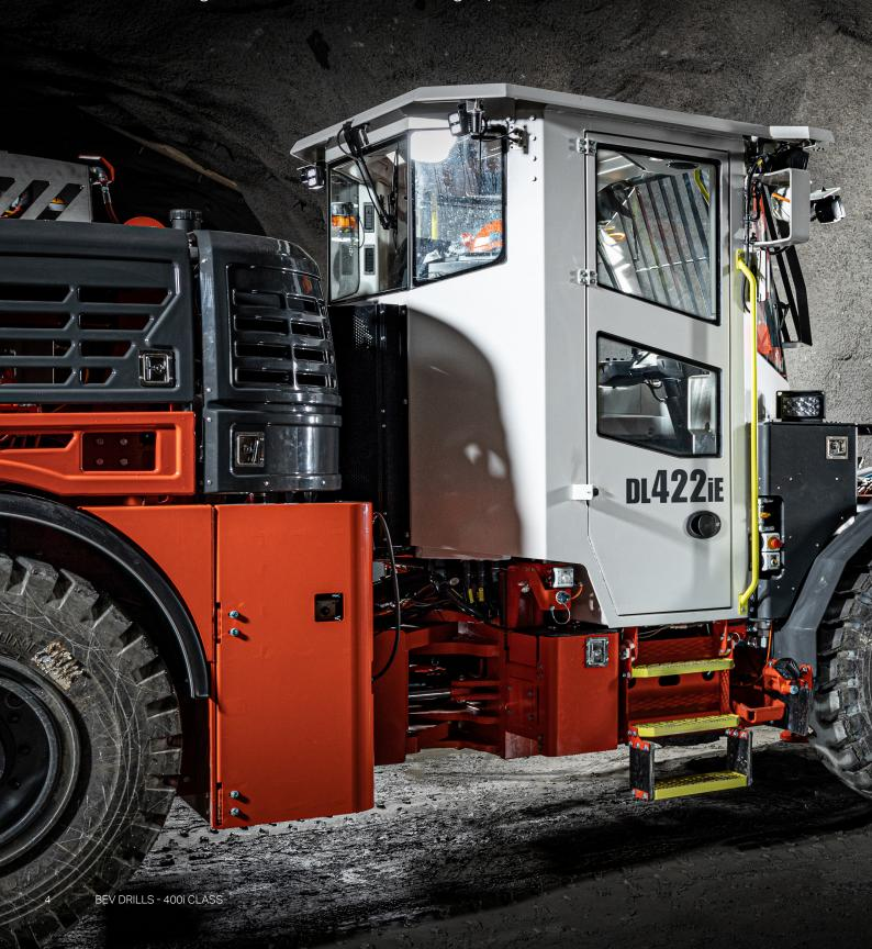
Equipped with the fully instrumented ZR35 telescopic boom, an automated rod handling system, and the powerful HF1560ST rock drill, Sandvik DL422iE provides accurate positioning, stability and accuracy in drilling for maximum performance.
