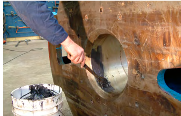
2. Clean the centre hole. Use a suitable solvent to remove the rust protection. Apply a lot of grease before fitting the stem.
