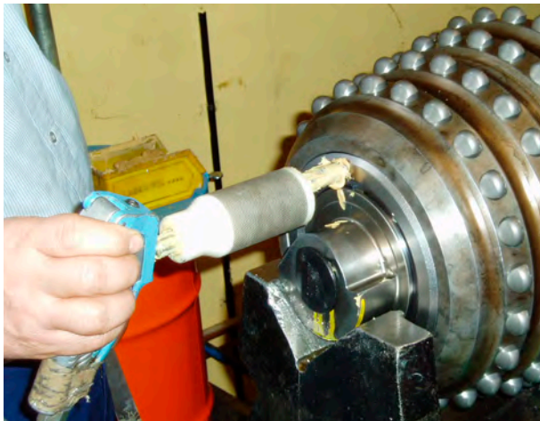
2. Attach a grease pump and start pumping.
