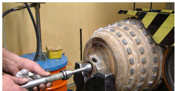
8. Re-install the ball plug retainer. Mount a new snap ring and a plastic protection cap together with new o-rings.
