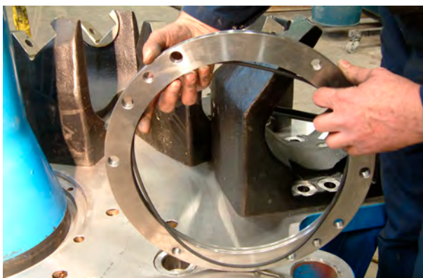
5. Clean the O-ring groove in the retainer ring and insert the O-ring.
