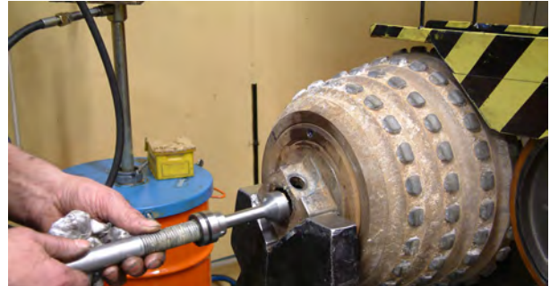
2. Pull out the ball plug retainer.
