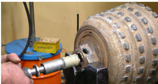
5. Clean the centre hole carefully. Install the re-greasing plug and attach the grease gun.
