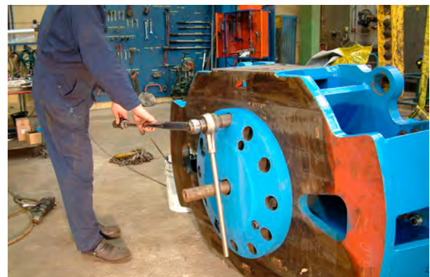
4. Push the stem into position. Oil the bolts. Pre-tighten the bolt crosswise to 800 Nm. Tighten to full torque 1200 Nm.
