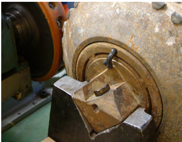
3. Continue to pump until grease comes out through the relief hole in the opposite seal retainer. Rotate the cutters \pm 20 revolutions. Mount two new conical plugs in each seal retainer.
