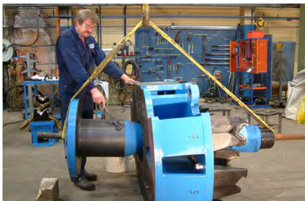
3. Insert the stem. Put a rod through the stem for easier handling. Clean and put a lot of grease on the inlet part of the stem. Use ordinary machine grease (0.5 kg).
