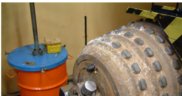
7. Rotate the cutter 20 revolutions. Continue to pump until grease comes out through the other relief hole. Mount a conical plug in this hole in the same way.
