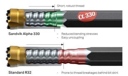
More steel for higher fatigue strength makes the connection rigid compared to the R32 to give exact collaring and straighter holes.
