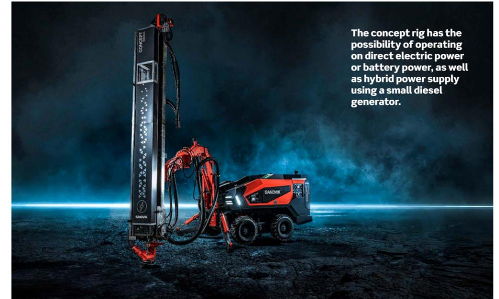
The concept rig has the possibility of operating on direct electric power or battery power, as well as hybrid power supply using a small diesel generator.
