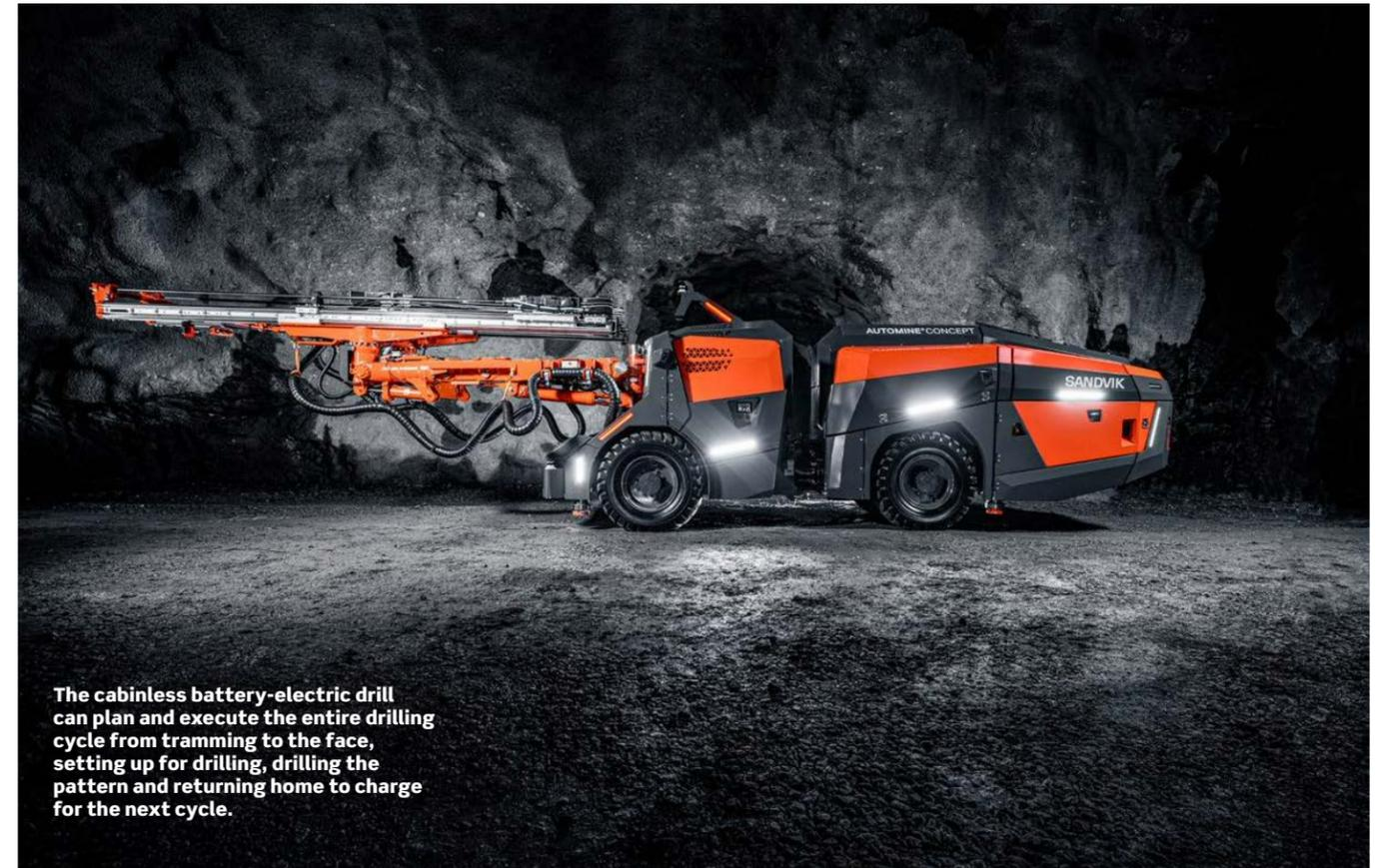
The cabinless battery-electric drill can plan and execute the entire drilling cycle from tramping to the face, setting up for drilling, drilling the pattern and returning home to charge for the next cycle.
