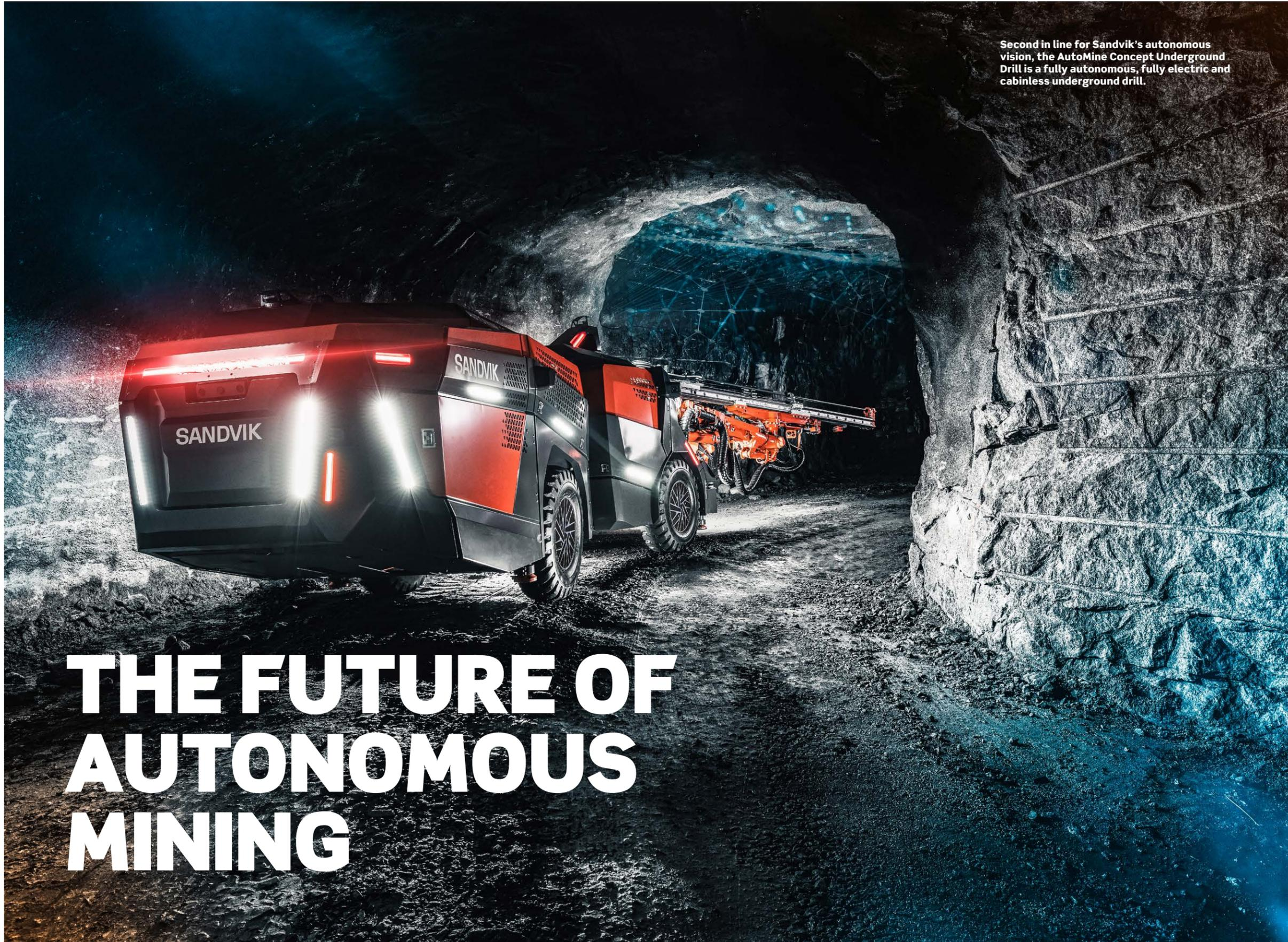
Second in line for Sandvik's autonomous vision, the AutoMine Concept Underground Drill is a fully autonomous, fully electric and cabinless underground drill.
