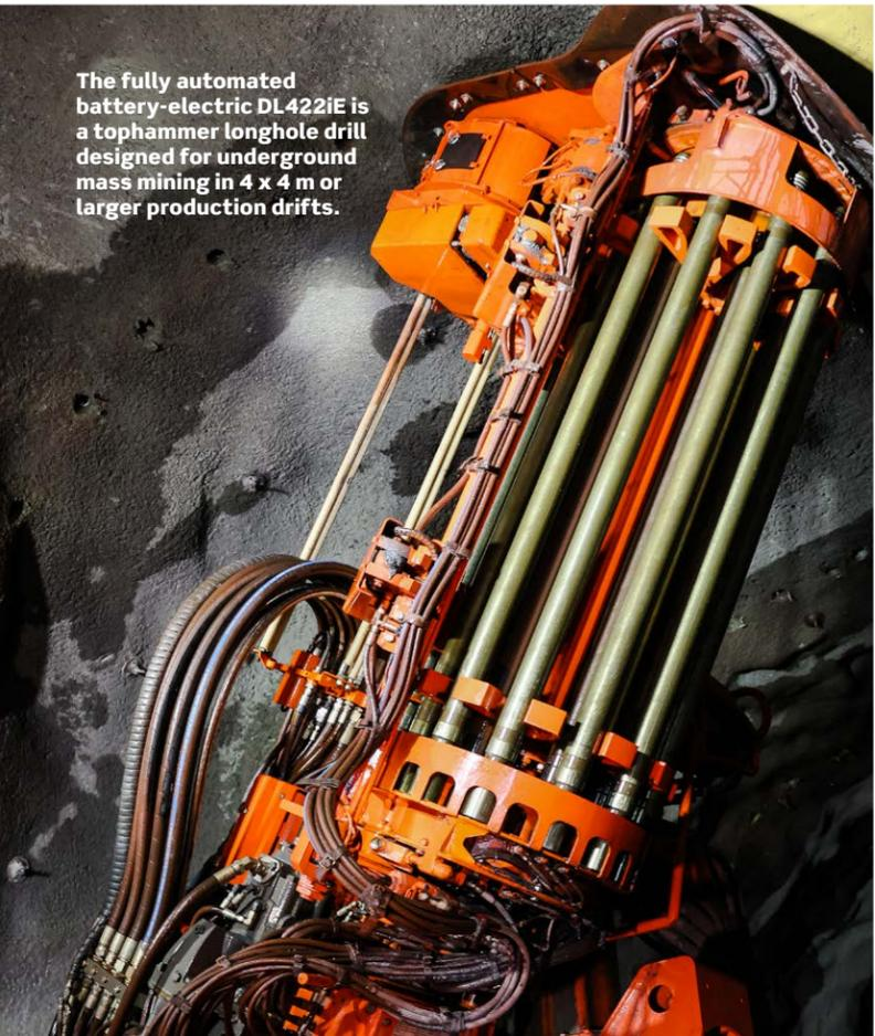
The fully automated battery-electric DL422iE is a topammer longhole drill designed for underground mass mining in 4 x 4 m or larger production drifts.
