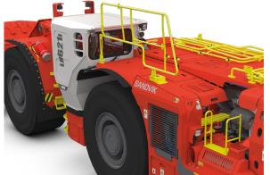
Separate battery and starter isolation switches are located at ground level access for troubleshooting while the engine is locked out for service.
