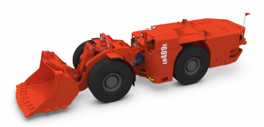
The LH409E is an electrically-driven loader for underground hard rock loading and hauling applications, with a tramming capacity of 9.6 metric tonnes. Reliability, fast bucket filling and rapid cycle times provide high capacity at low cost per tonne. The LH409E fits in an evelope of 3.5 m x 3.5 m.
