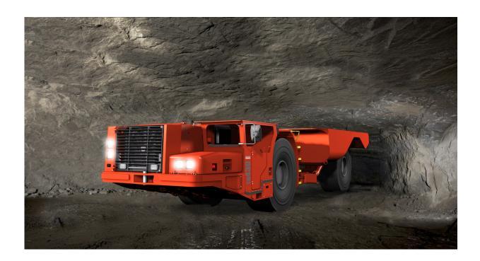
Sandvik TH430L is a 30 metric tonne articulated low profile dump truck that will fit in a 4 x 2 m envelope.
